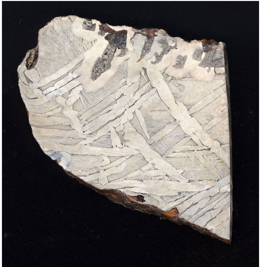
Widmanstätten pattern on a fragment of the Seymchan meteorite found in the Magadan district of Russia in 1967. Courtesy Basilofresco, licensed under Creative Commons .
