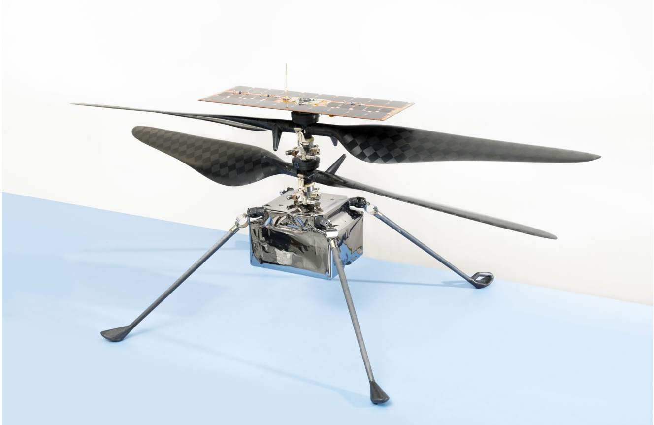
The flight model of NASA's Ingenuity Mars Helicopter. Credit: NASA/JPL-Caltech
