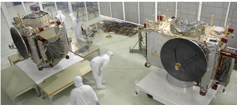
NASA'S dual STEREO spacecraft, whose mission is the first to take measurements of the sun and solar wind in 3-D, are seen undergoing final preparation within the clean room at Astrotech, a processing facility near Kennedy Space Center during May 2006. Courtesy NASA/Jim Grossmann.
